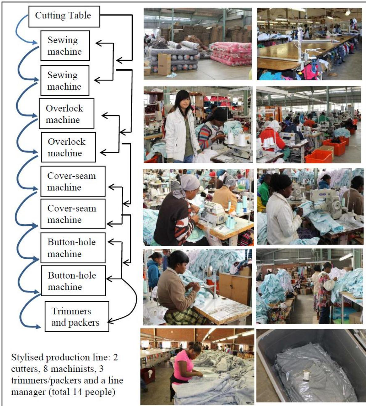
Figure 10: A labour intensive production line (basic items).
